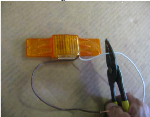
Cut approximately 8 1/2" off of the white wires on both running lights.
