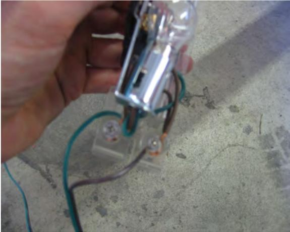
Loosen the wire retaining screws and install the color matching wires from the wire harness onto the corresponding retaining screws.
