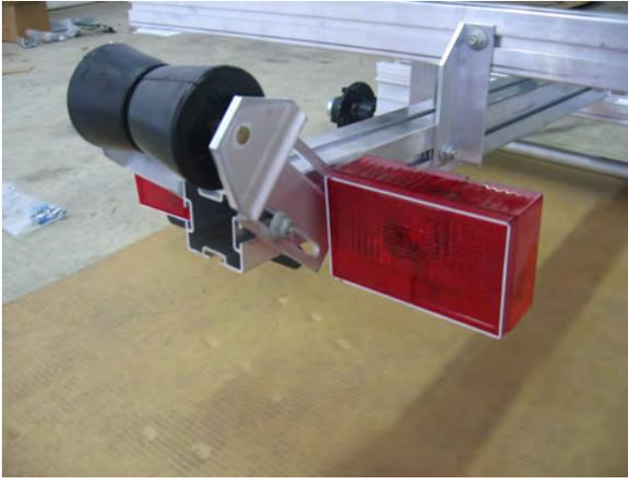
Repeat this procedure to install the right tail light onto the right tail light bracket.
