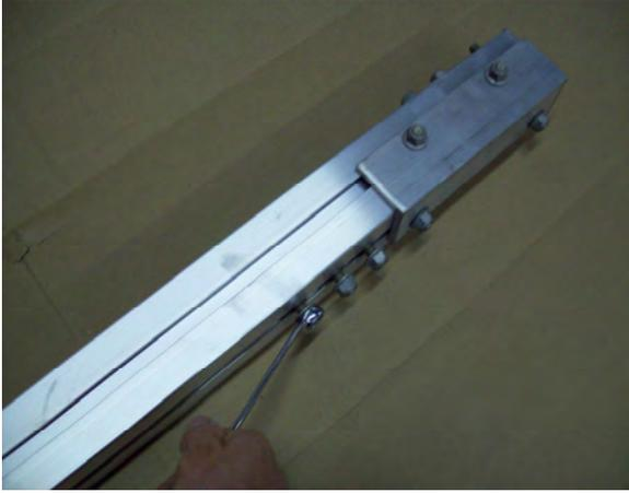
Unwrap the two tongue sections and loosen the 6 nuts (3 per side) located at the rear of the front tongue section and slide them all the way forward toward the coupler. These will be used later to install the front cradle and the bow stand.
