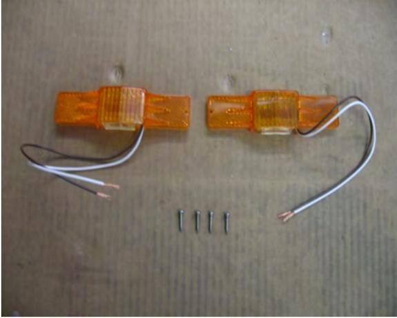
Locate the two amber running lights and four small Philips screws.
