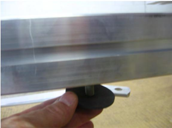
Install the rubber washer that was removed previously onto the 1 1/8" T-bolt located in the bottom slot approximately 72" from the rear.
