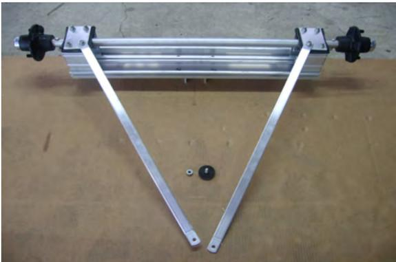
Rotate both tie rods forward.
