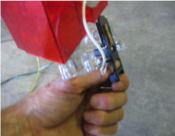
Move the tab toward the rear of the trailer and pull down releasing the bulb assembly from the light housing.
