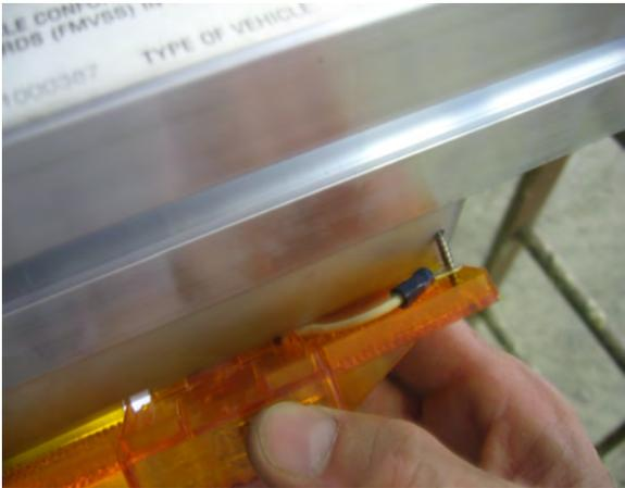
Install the running lights into the pre-drilled holes in the running light bracket using a Philips screwdriver. Be sure the screw is through the ring terminal on the back side of the lights. This will supply a ground to the lights. DO NOT OVER TIGHTEN.
