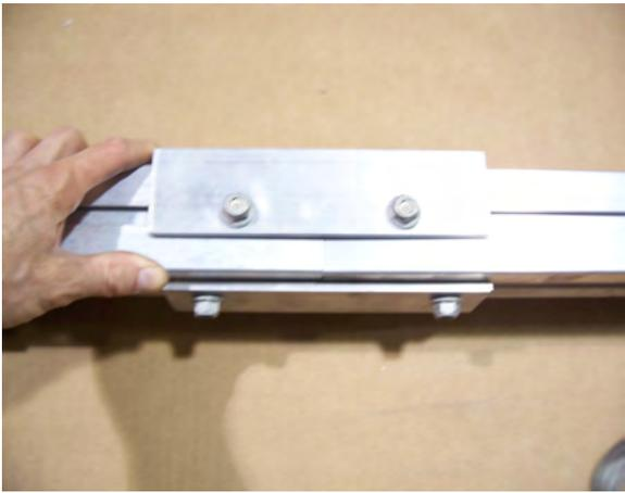
Slide each plate over the adjacent tongue section until the plates are centered over the gap between the tongue sections.
