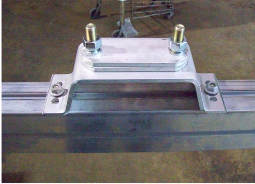
Position carrier about 12" away from the splice plates then tighten nuts.
