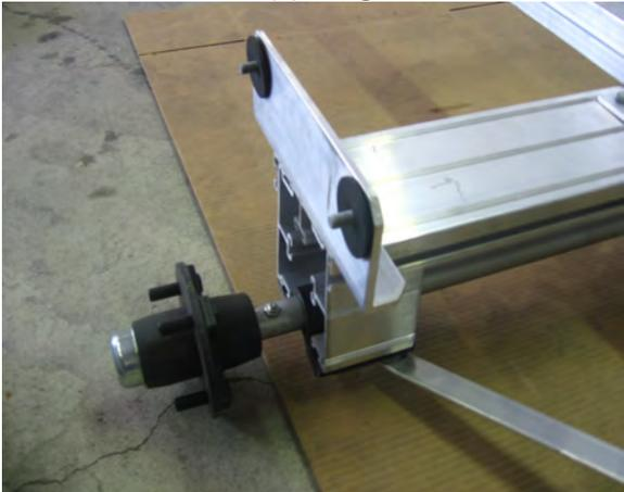
Install the 1" bolts and (2) rubber washers as shown.
