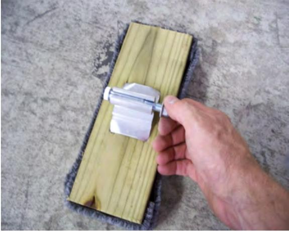
Remove the bolt from the pivot plate.
