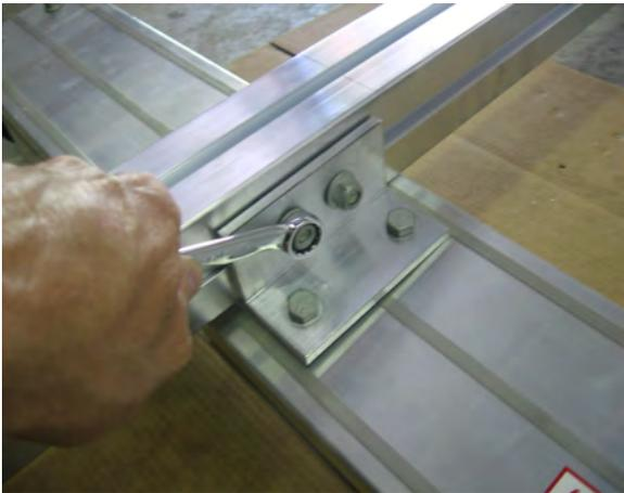
Go back and tighten all the nuts that attach the tongue to the axle.
