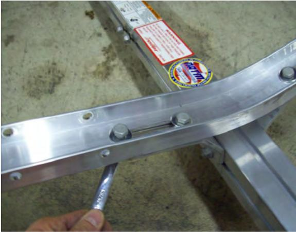
Slide the bolts out to the ends of the slots and tighten the nuts.
