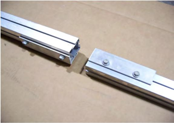
Lay the tongue sections end to end with the splice plates adjacent to each other. Loosen 4 nuts on each splice plate.
