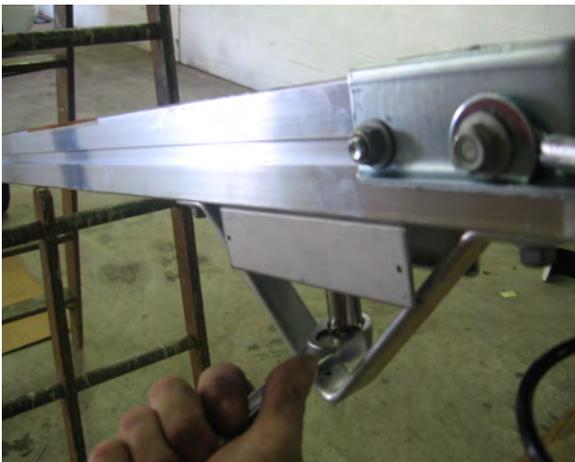
Tighten the nuts for the skid and running light bracket in the location shown.
