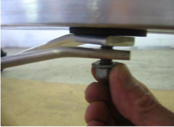
Install the forward ends of both tie rods to the 1 1/8" T-bolt. This will ensure that the axle assembly is perpendicular to the tongue.
