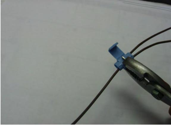
(Illustration) Use pliers to push the metal spade down until it is flush with the plastic. This is what makes the electrical connection between the two wires.
