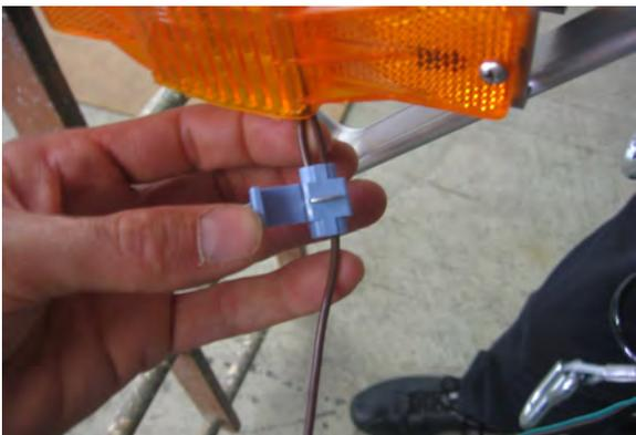
Pass the brown wire from the other running light through the remaining open slot in the connector at a point close to the running lights.
