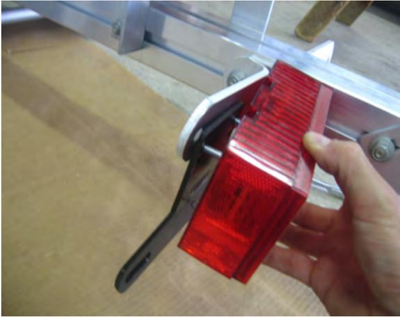
Install the license plate bracket and left tail light onto the tail light bracket.
