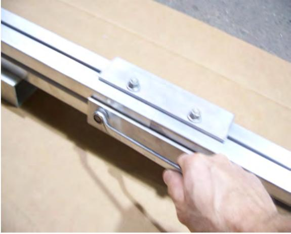
Tighten all 8 nuts making sure that the tongue sections are as tight as possible to one another. Set the tongue aside.
