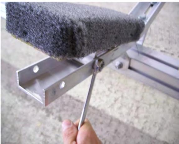
Install the padded cradle (inner position shown – this may vary depending on the width of the hull). Final angle will be determined when the trailer is fitted to the boat.
