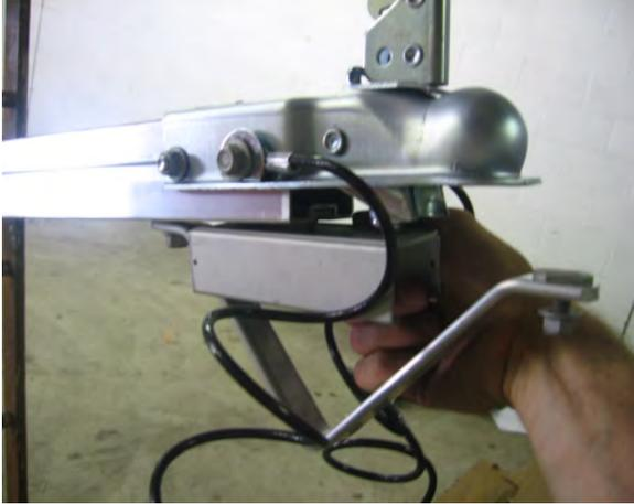
Slide the running light bracket into the bottom slot in the front tongue section.
