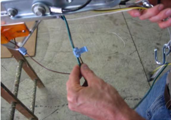
Measure 22" back from the front plug on the green/brown wire and pass the brown wire through the open slot in the second light blue connector at this location. The green wire will rest just outside the connector. Insert the brown wire from the running lights into the closed side of the connector and close the spade and cover as previously described. This will make the connection from the main harness to the running lights.
