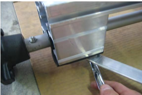
Important! Tighten the nuts at both ends of the tie rods.
