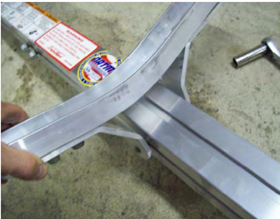
Using the rearward most bolts of the three that were moved toward the coupler during tongue assembly, attach the front cradle holder assembly at the pencil marks located 36" from the front of the tongue. Final location of the front cradle holder will be determined when the boat is fitted to the trailer.
