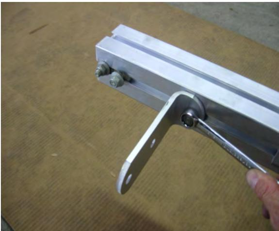
Install the tail light brackets loosely and slide them toward the front of the trailer - final location to be determined later.
