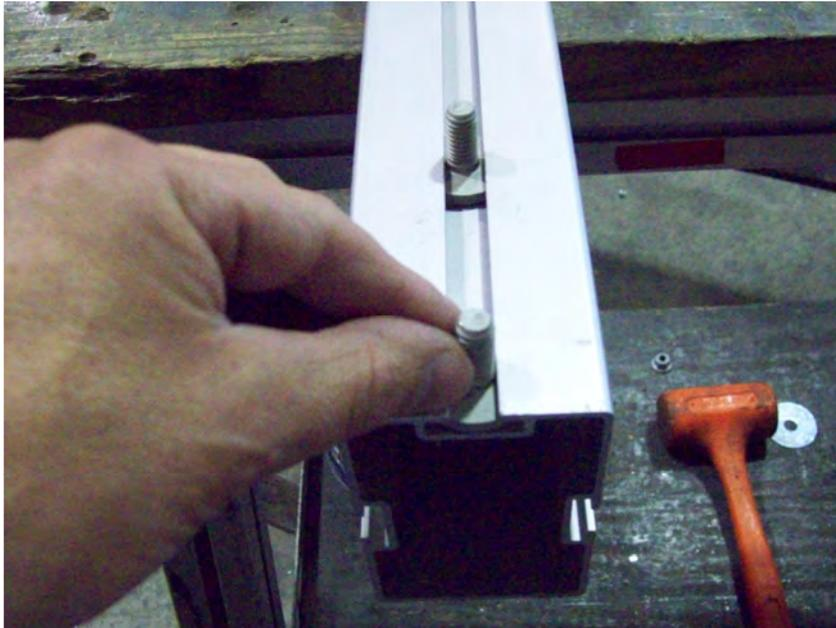
Slide 2 T-bolts on the underside of the front tongue section that has the serial number on it.
