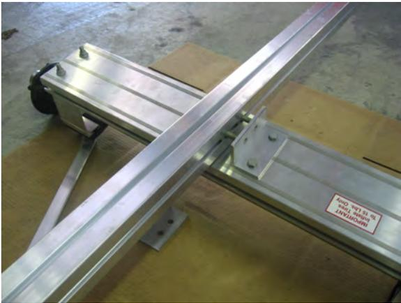
Attach the tongue section to the axle assembly with the tie rods facing forward. Align the rear edge of the axle assembly with the pencil line on the bottom of the tongue section located at 42" from the rear.
