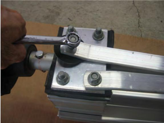
Remove the 1 1/8" T-bolt and rubber washer located on the tie rod end and set them aside for installation later.
