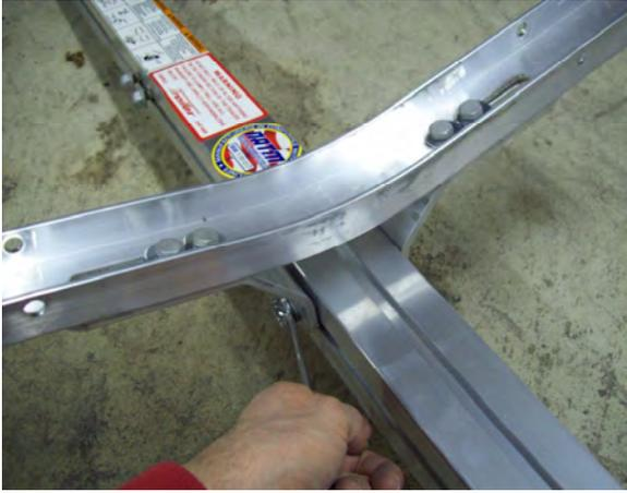
Tighten the nuts making sure the cradle holder brackets are perpendicular to the tongue.
