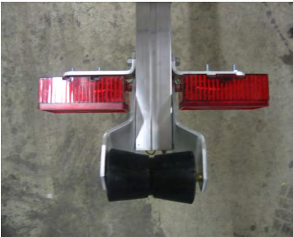
Loosen the tail light brackets, slide them to the rear as far as possible and tighten the nuts.
